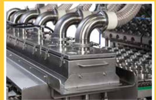
XENON's washdown Pulsed Light housing for installed on a yogurt filling line manufactured by Alfa Machine.
