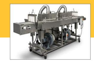
PUV light treatment achieved up to 5 log microbial reduction on food contact surfaces using a XENON Pulsed Light RC-802 Interweave system.
