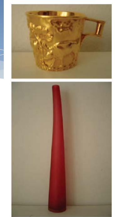
Metallic gold and gold nanoparticles in ruby glass
