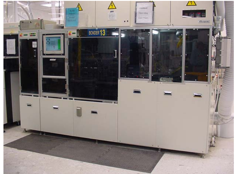
The automated DVD Bonder at WAMO used pulsed UV, high peak power tests in the year 2000.
