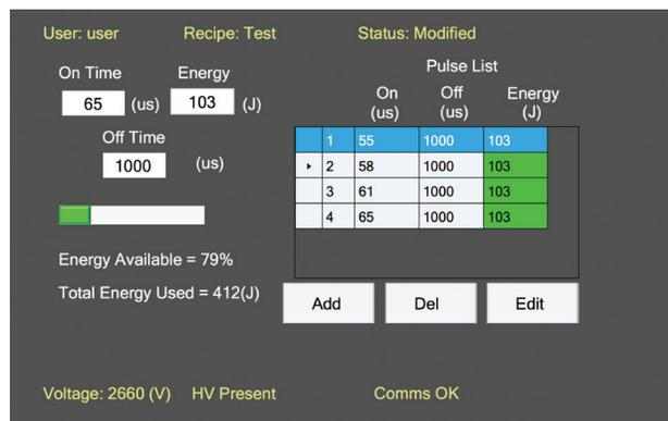
Programming pulse profiles and sequencing is done on a single screen.
