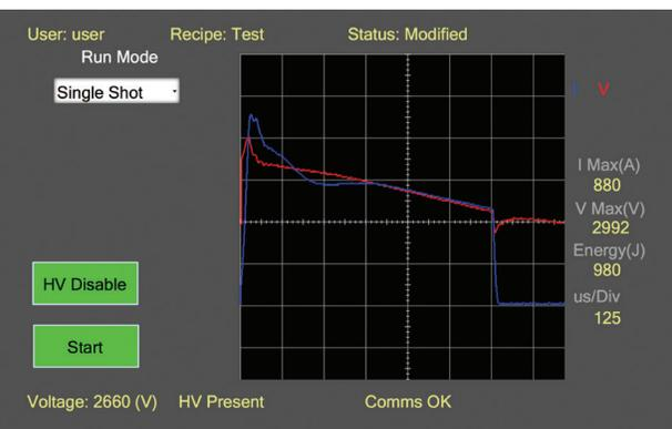
Lamp operating parameters (voltage and current) and pulse energy are monitored and displayed to confirm system operation.
