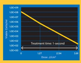
Destruction of B. subtilis in suspension exposed to Pulsed Light. Reduction of >6 log CFU/ml achieved within 1-second treatment time.
