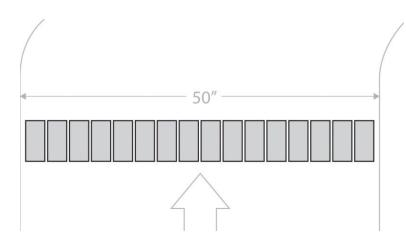
[Figure 2 Caption] Lamps parallel to printing line: up to 16 required to span press width
