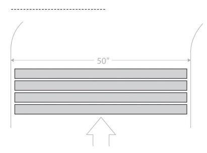
[Figure 3 Caption] Lamps axial to printing line: one lamp system spans the full width
