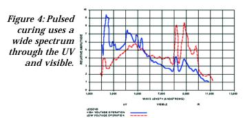
The chief virtue is the degree of control this affords the user. Processes can happen, stop - start - stop - start, with the pressing of a button or sending of an electronic signal from a programmable logic controller (PLC). For DVD makers, the important benefits are that since the substrate is at a lower temperature, it is less likely to warp like a potato chip and the lamp has a longer lifetime. This leads to better quality, higher yields, and lower operating costs.
