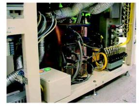
Figure 7: Some pulsed UV lamps have compact power supplies, which help minimize the footprint of an automatic bonder.
