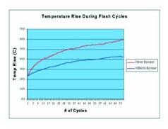
Figure 3: Temperature rises at glass surface vs. cycles of minimum required flashes.
