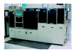
Figure 1: An automated DVD bonder, at the WAMo facility in Pennsylvania uses pulsed curing.
