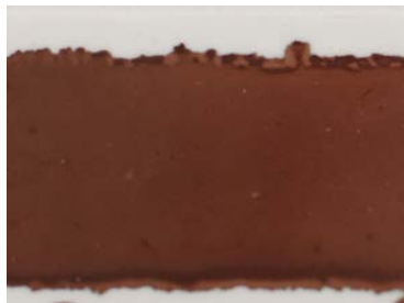
Thin Copper on Alumina
