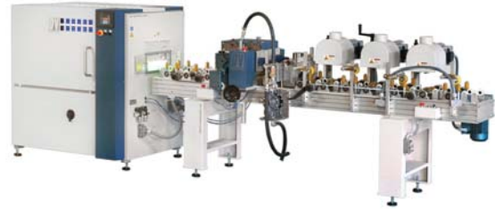
Figure 9: UV Roll-Coat System
